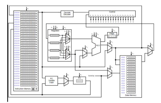
This is the data flow of the I281 CPU. The data flow consists of decoding instruction memory, changing control signals, and doing arithmetic. This visual provides the general layout of the I281 CPU, with lines that demonstrate the paths and connections that are needed between each component.
